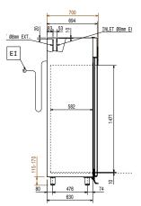
Electrical inlet (power) RI Refrigerant Inlet Refrigerant Outlet
